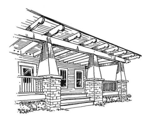
fig. 25. Porch and Exposed Structural Supports
